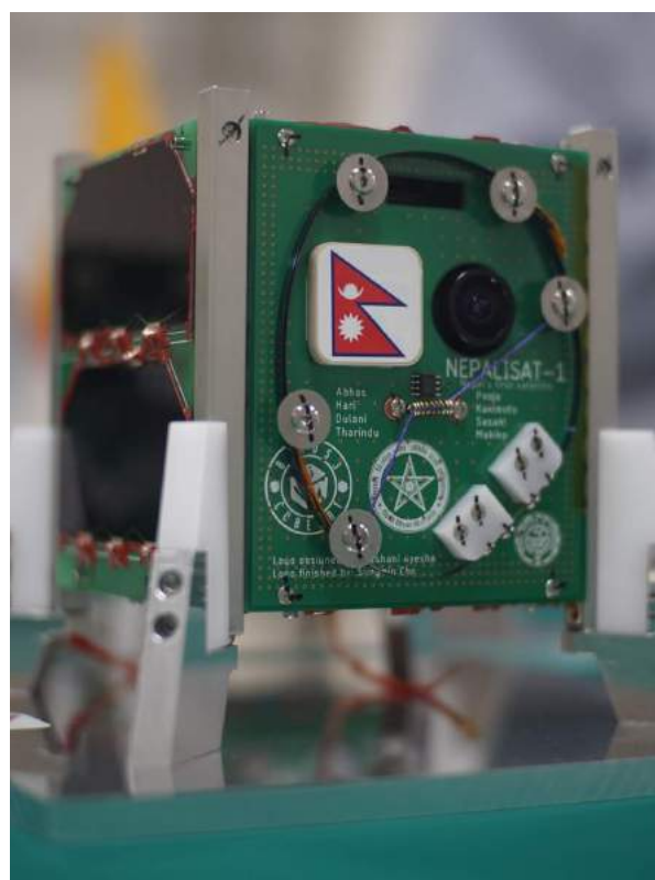
The NepaliSat - 1 is a cube satellite which weighs about 1.3 kg. The satellite clicks geographical pictures of Nepal.
